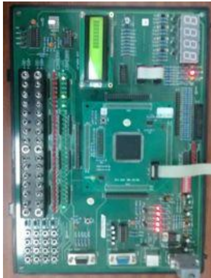
Fig 3 FPGA image showing coin detection by LED's
